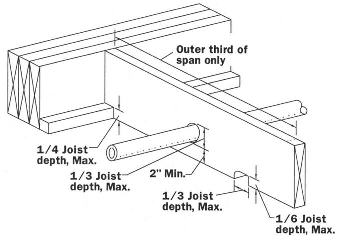
Figure 4.—Joist and rafter notching and boring limits.
