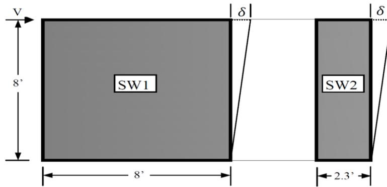
Figure 5. Distribution of shear to shear walls in a line to produce equal deflection in each shear wall is the underlying basis of the familiar  $2b_s/h$  factor
