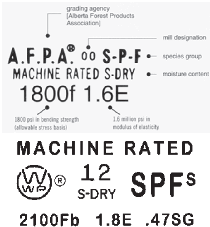
Figure 1.—A typical MSR grade stamps. The bottom figure shows a specific gravity value.
