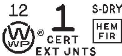
Typical grade stamp for certified finger-jointed lumber.
