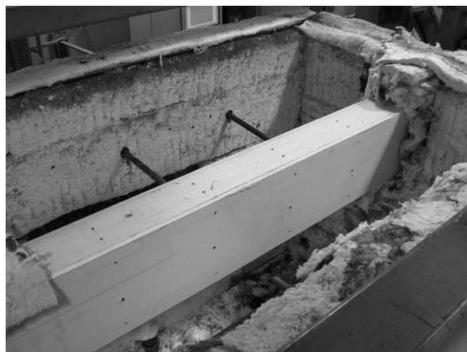
**Figure 1.**—Specimen in intermediate-scale horizontal furnace.
