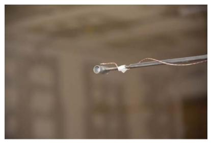
Figure 80. Bidirectional probe.
