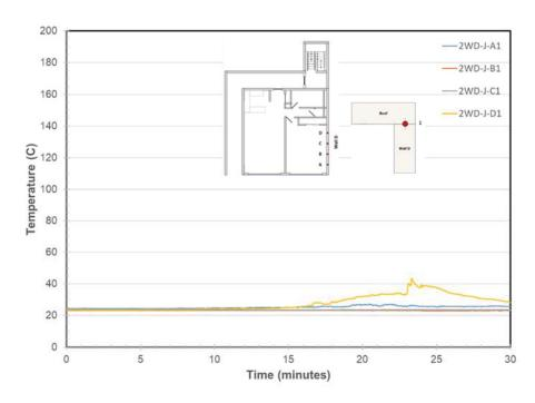
Figure 32. Ceiling/Wall B Joint Temperatures at Locations A-D
