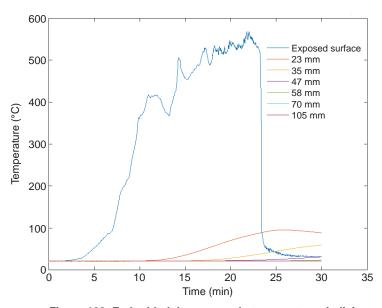
Figure 108. Embedded thermocouple temperatures in living room wall at Location B for Test 5.
