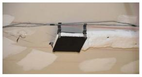
Figure 84. Directional flame thermometer mounted on ceiling.
