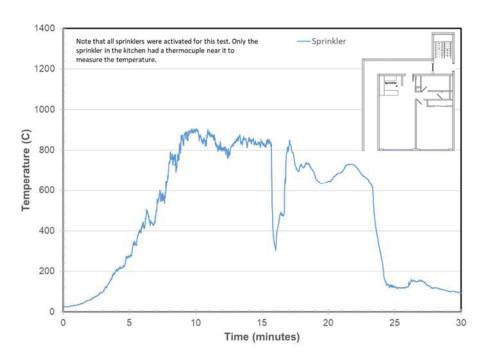
Figure 16. Sprinkler Head Temperature in Kitchen
