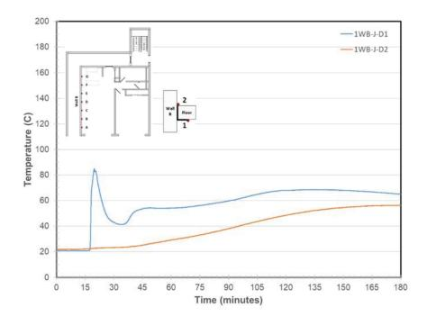
Figure 943. Wall B/Steel Angle Joint Temperatures at Location D
