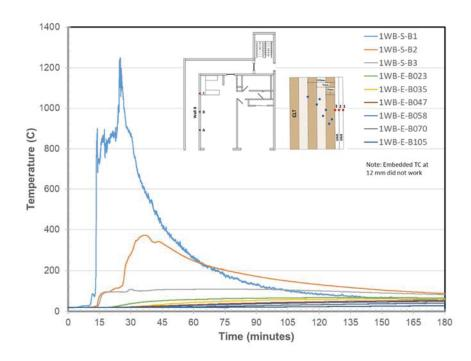
Figure 924. Wall B Embedded & Surface Temperatures at Location B
