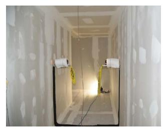
Figure 90. Optical density meters located in the corridor.
