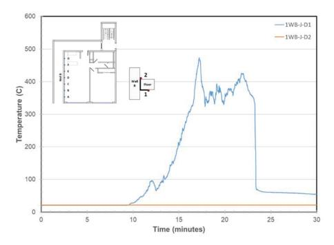
Figure 23. Wall B/Steel Angle Joint Temperatures at Location D
