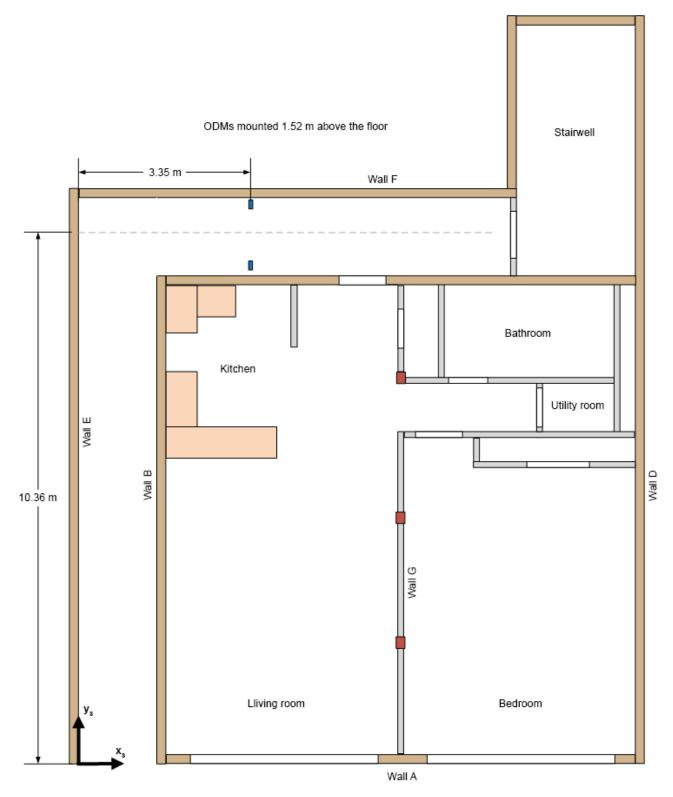
Figure 91. Location of optical density meters (ODMs) (blue rectangles).
