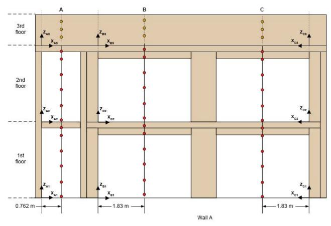
Figure 78. Location of thermocouples on Wall A (red and yellow circles).
