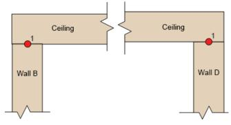
Figure 75. Ceiling—wall joint temperature measurement locations (second floor).
