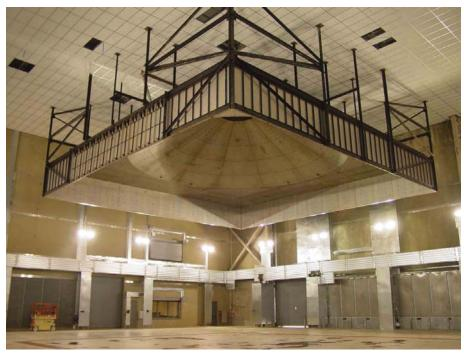
Figure 96. 14-MW fire product collector at the Bureau of Alcohol, Tobacco, Firearms and Explosives (ATF) Fire Research Laboratory.
