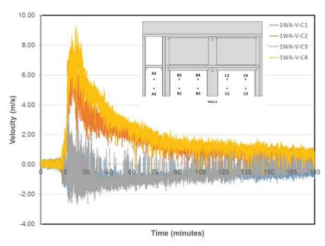
Figure 957. Velocity at Location C on Wall A
