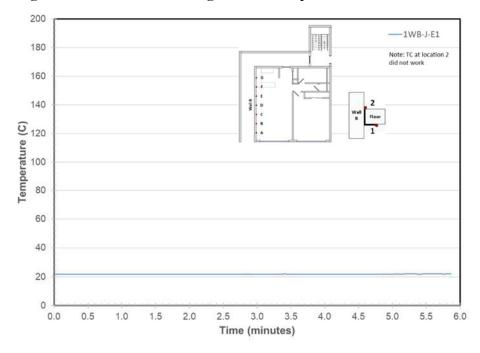
Figure 253. Wall B/Steel Angle Joint Temperatures at Location E
