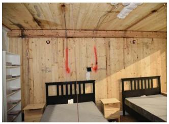
Figure 37. Exposed ledger in the bedroom for Tests 4 and 5.
