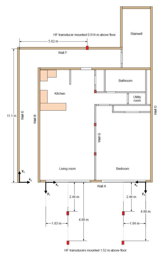
Figure 83. Location of heat flux (HF) transducers (red rectangles).
