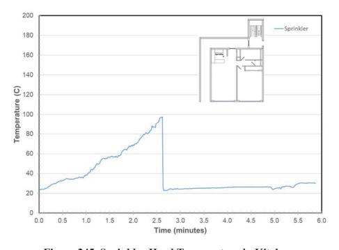
Figure 245. Sprinkler Head Temperature in Kitchen
