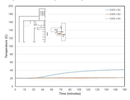
Figure 948. Wall D/Ledger Joint Temperatures at Location B
