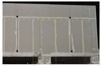
Figure 88. Directional flame thermometers mounted on the exterior of Wall A.  $\begin{tabular}{ll} \hline \end{tabular}$
