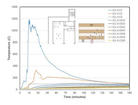
Figure 927. Living Room Ceiling Embedded & Surface Temperatures at Location C
