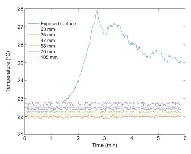
Figure 107. Embedded thermocouple temperatures in living room wall at Location B for Test 4.
