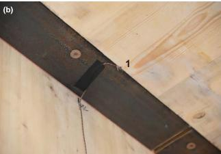
Figure 72. Thermocouples placed between the steel angle and the cross-laminated timber floor assembly to measure the joint temperatures: (a) top view; (b) bottom view (numbers correspond to locations shown in Fig. 71).
