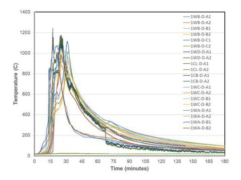
Figure 953. DFT Temperatures at each Location on 1st floor
