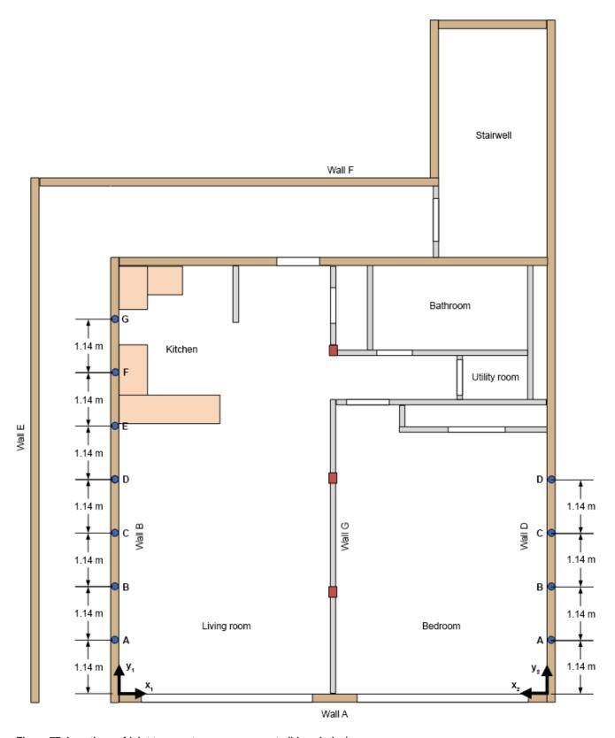
Figure 77. Locations of joint temperature measurements (blue circles).
