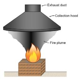
Figure 95. Schematic of a fire product collector.
