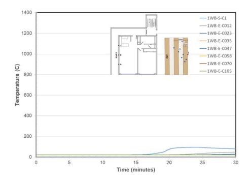
Figure 4. Wall B Embedded & Surface Temperatures at Location C
