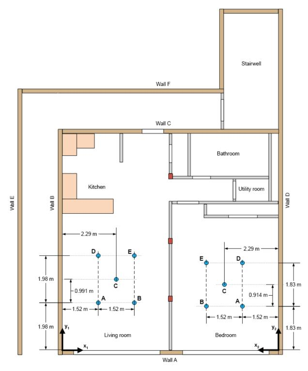
Figure 67. Location of ceiling thermocouples (blue circles).
