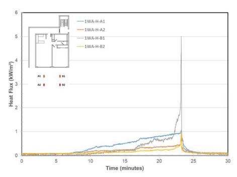
Figure 37. Heat Fluxes in Front of Wall A
