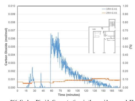
Figure 966. Carbon Dioxide Concentrations in the corridor on each Floor
