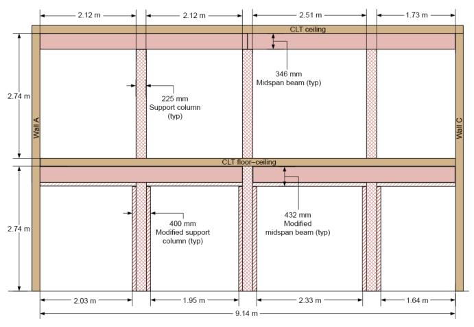
Figure 14. Cross-sectional view of apartment showing locations of support columns.
