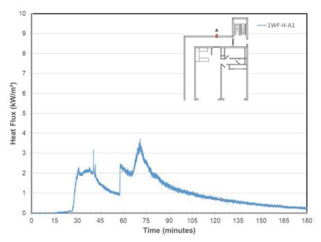
Figure 959. Heat Flux on Wall F across from Apartment Door
