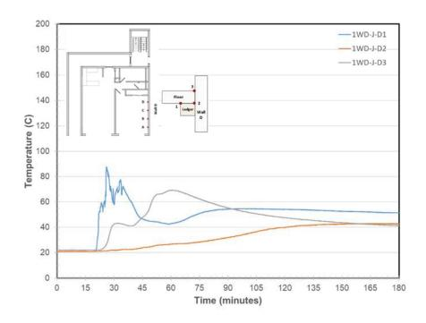
Figure 950. Wall D/Ledger Joint Temperatures at Location D
