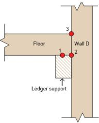
Figure 73. Ledger–floor joint temperature measurement loctions.
