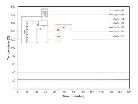
Figure 951. Ceiling/Wall B Joint Temperatures at Locations A-G
