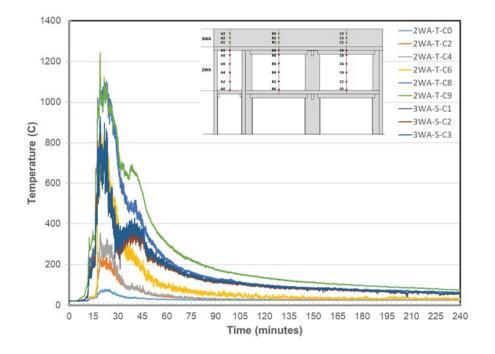
Figure 18. Wall A Temperatures at Locations C
