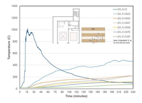
Figure 6. Living Room Ceiling Embedded & Surface Temperatures at Location C
