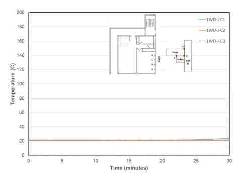
Figure 29. Wall D/Ledger Joint Temperatures at Location C
