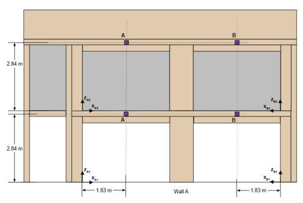
Figure 89. Location of directional flame thermometers on Wall A (purple squares) (see also photograph in Fig. 52).
