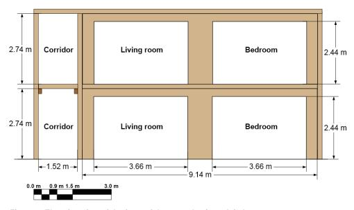
Figure 2. Elevation view of the front of the cross-laminated timber test structure.
