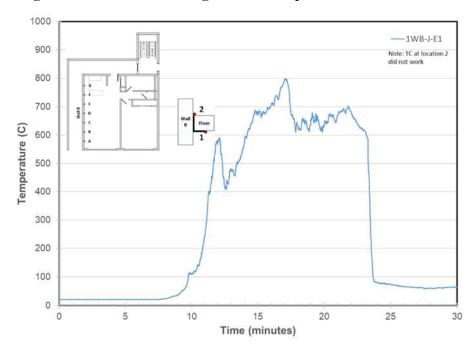
Figure 24. Wall B/Steel Angle Joint Temperatures at Location E
