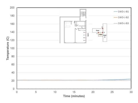
Figure 28. Wall D/Ledger Joint Temperatures at Location B
