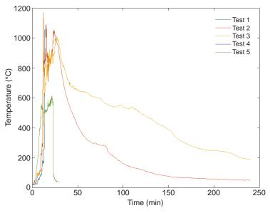
Figure 102. Living room air temperature at 1.83 m above finished floor at location B for each test.
