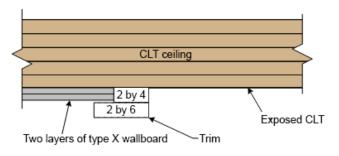
Figure 34. Trim added to exposed cross-laminated timber ceiling to protect edge of gypsum wallboard.
