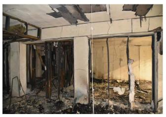
Figure 58. Interior view of apartment after Test 1.
