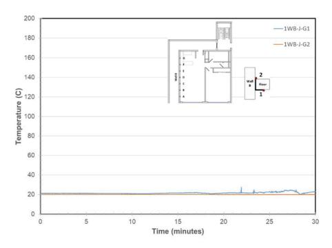
Figure 26. Wall B/Steel Angle Joint Temperatures at Location G
