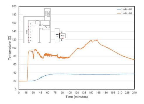
Figure 20. Wall B/Steel Angle Joint Temperatures at Location B
