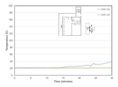
Figure 21. Wall B/Steel Angle Joint Temperatures at Location B
