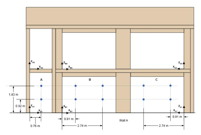
Figure 81. Location of bidirectional probes (blue circles).
