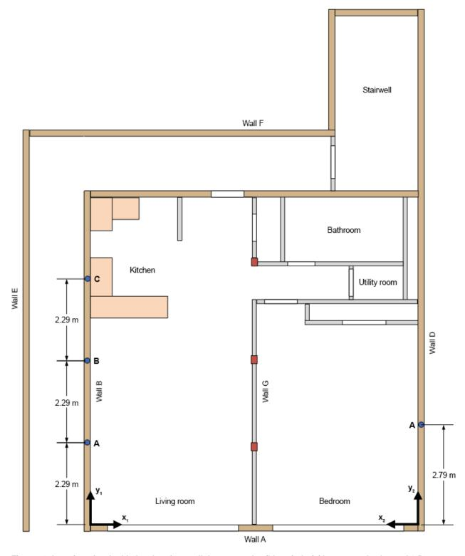
Figure 70. Location of embedded and surface wall thermocouples (blue circles) (thermocouples located 1.52 m above the finished floor).
