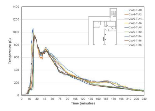
Figure 14. Wall G Temperatures at Locations A & B
