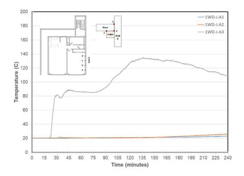
Figure 26. Wall D/Ledger Joint Temperatures at Location A
