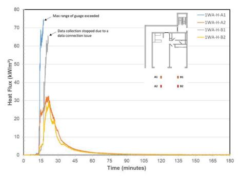
Figure 958. Heat Flux in Front of Wall A
