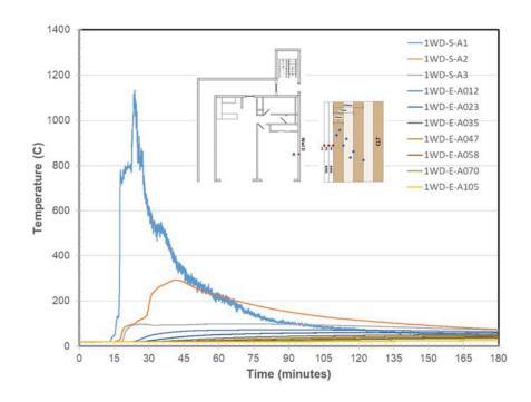
Figure 926. Wall D Embedded & Surface Temperatures at Location A
