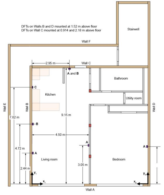
Figure 85. Location of directional flame thermometers (DFTs) on interior walls (purple rectangles).
