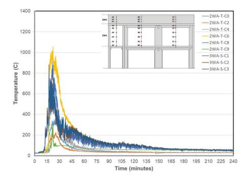
Figure 223. Wall A Temperatures at Locations C
