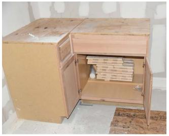
Figure 51. Ignition package located inside of kitchen cabinet.
