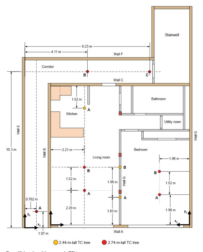
Figure 66. Location of thermocouple (TC) trees.
