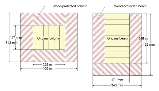
Figure 15. Cross-sectional view of a support column and midspan beam illustrating the wood protection added to achieve a 2-h fire resistance rating.
