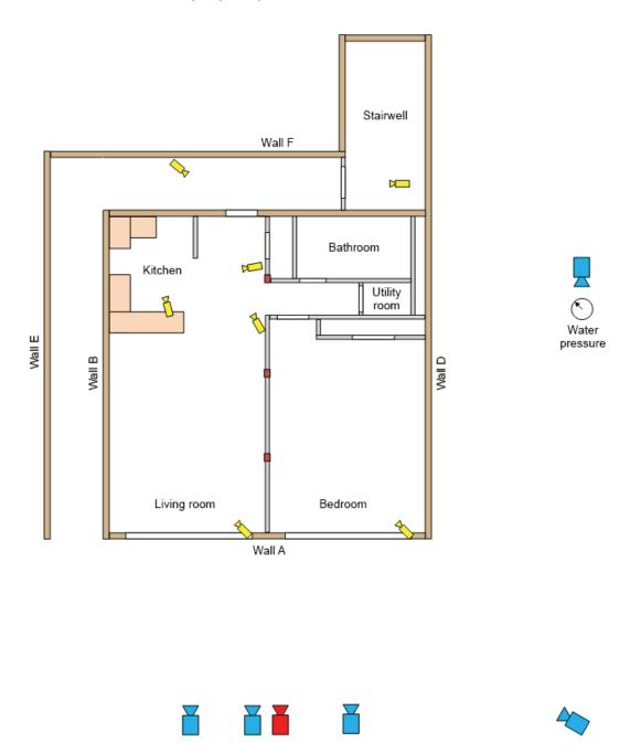
Figure 97. Layout of video cameras (HD, high definition; FLIR, forward looking infrared radiometer; SD, standard definition).
