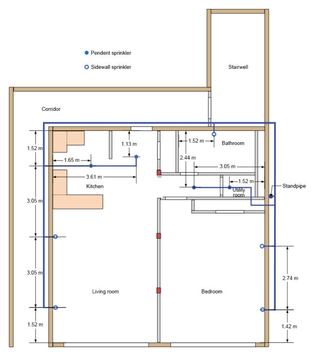
Figure 41. Sprinkler layout.
