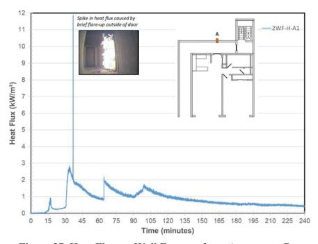
Figure 37. Heat Flux on Wall F across from Apartment Door
