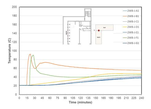
Figure 30. Ceiling/Wall B Joint Temperatures at Locations A-G
