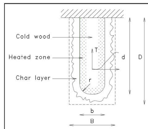
Figure 12: Heavy Timber Member Exposed to Fire
