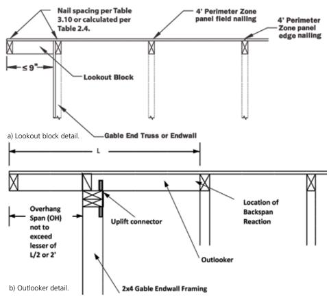
Figure 4. Rake overhang outlooker and lookout block details (excerpted from 2018 WFCM).
