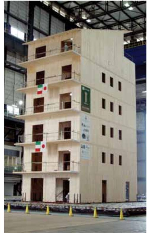
Seven-story CLT building being tested on the world's largest shake table in Miki, Japan
